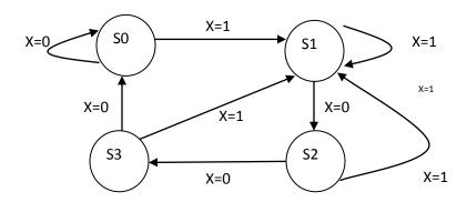
(b) (10 points) Draw the next-state table, and derive the functions for D1 and D0. Derive the output function.
