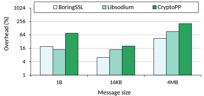
Fig. 7: Encryption overhead (256-bit key), drawn in log scale, for Encrypted_Bcast on Ethernet.
